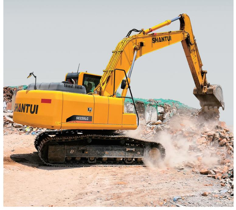
Engine Model: Cummins B5.9-C Gross Power: 112 kW/1950 rpm
